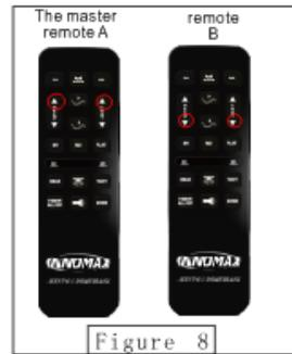
To desynchronize the clone remote(B) from master remote(A) ,press the **▲▲** and **▼▼** buttons of the clone remote(B),the desynchronizing process is successful when the clone(B) flash light normally on.(See figure 9)
